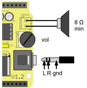
can power the amplifier with a higher voltage ( up to 18 volts ) through the use of the external power jack on the Arduino board.
