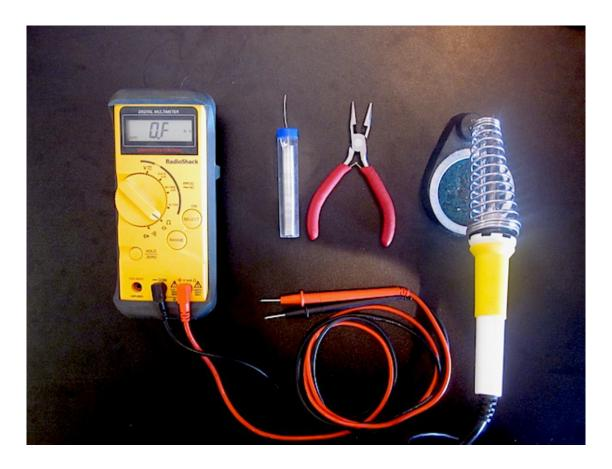
The GinSing hardware requires only a couple of tools and basic soldering skills. You will need to have a good working **soldering iron**, **solder**, and **side cutter** | needle nose **pliers** If you are just starting out we highly recommend this <u>beginners toolkit</u>.
